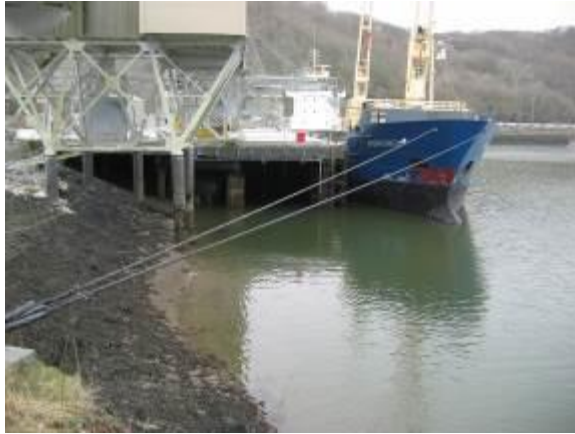
long ships head lines are run from the ship to a shore point on an embankment by boat
