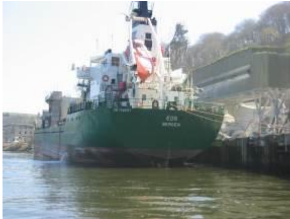
long ships head lines are run from the ship to a shore point on an embankment by boat
